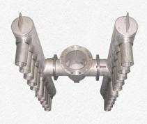
The Pipe Type Distributor is a straightforward design that can be highly effective when there is a high vapor flow. Its simple construction with pipes allows for a large volume for the vapor to flow through.
