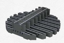
The liquid distributor LO features troughs with lateral notches serving as discharge openings. These troughs are supplied by a parting box, making this distributor highly resistant to fouling and broadening its range of applications. A trough type distributor includes a pre-distribution opening, also known as a 'parting-box,' positioned above several evenly spaced narrow troughs.
